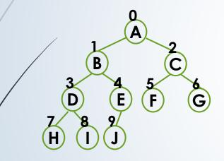
We can represent binary trees using array by applying this numbering scheme.
