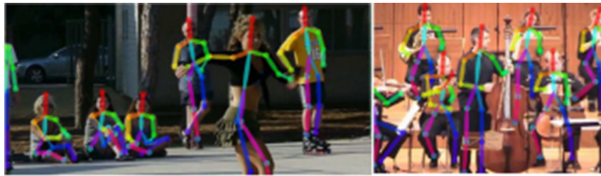
Figure 2: Human skeleton keypoint recognition (OpenPose) [28]
