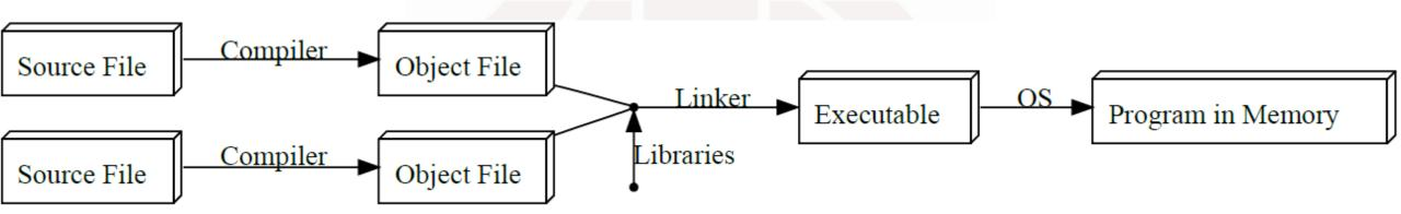
• **Object file**: intermediate file that represent an incomplete copy of the program, each source file only expresses a piece of the program, so when it is compiled into an object file, the object file has some markers indicating which missing pieces it depends on.
