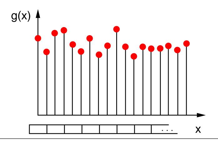
Reconstructed signal (again by fitting a smooth function to it)
