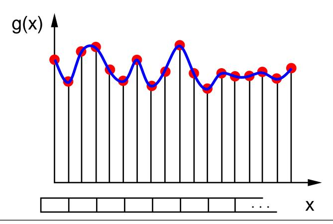
Reconstructed signal superimposed on original signal
