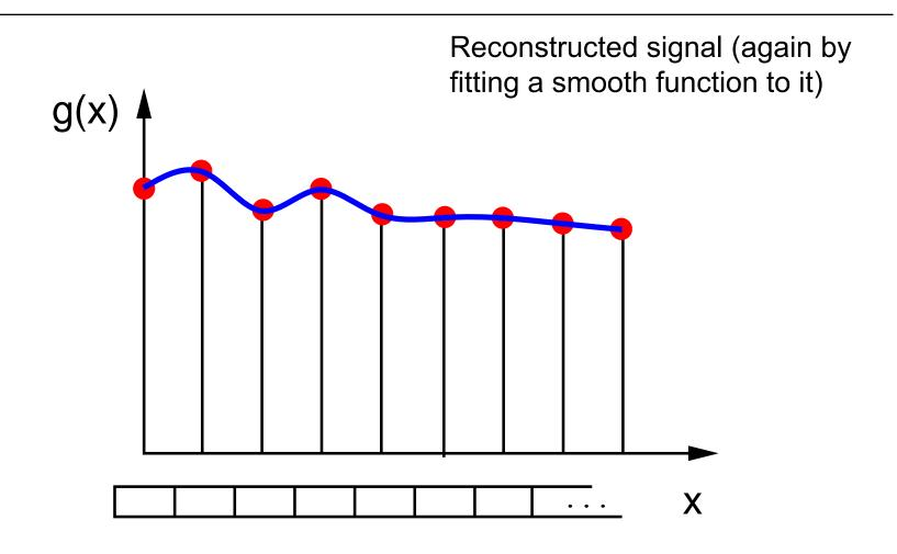
Reconstructed signal superimposed on original signal
