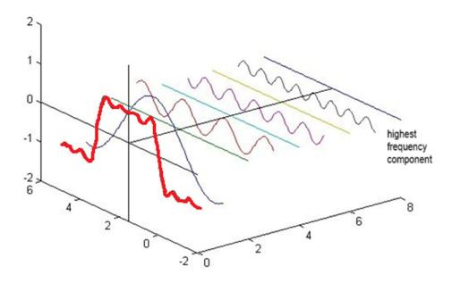
A 1D audio signal (e.g., the red curve) can be decomposed into many basic frequency components (four in the above example). The highest frequency component  $f_h$  of this audio signal is the right most one.
