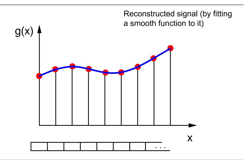
Reconstructed signal superimposed on original signal
