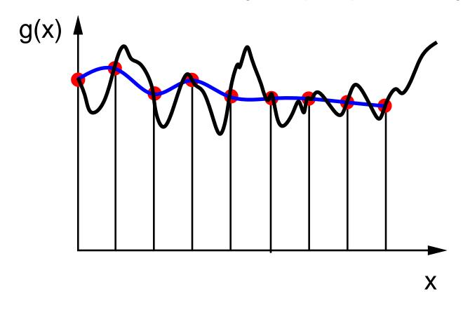
Now, if we reduce the sampling interval,  $\Delta x$ , by half (i.e., doubling the sampling rate) as follows:
