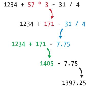
Figure 2-1: The order of operations: multiplication, division, addition, subtraction
